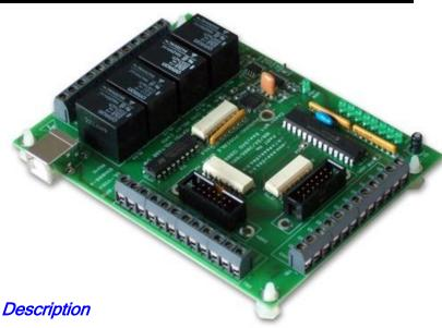
Low cost, general purpose, USB connected & powered, 8 channel voltage input, 4 channel DIO and 4 channel relay card. Voltage input and relay channels are opto-isolated.
